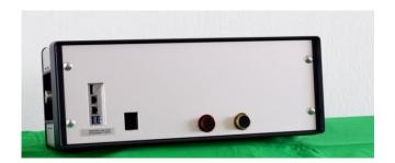
On the back panel, 2 USB ports are available to connect a printer, keyboard or mouse.
