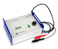
The low supplied current (0,3mA) prevents the destruction of the cable in case of default. The fault is indicated by the variable lighting of the lamp, flashing when the current leakage reaches  $10\mu A$ .
